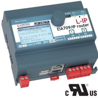
The L-IP Routers LIP-1ECTC, LIP-3ECTC, LIP-33ECTC, and LIP-3333ECTC connect twisted pair channels (TP/FT-10 or TP/XF-1250) with the Ethernet/IP channel (IP-852) in LonMark Systems. L-IP routes CEA-709 packets through an IP based network such as a LAN (Ethernet), an Intranet, or even the Internet.
