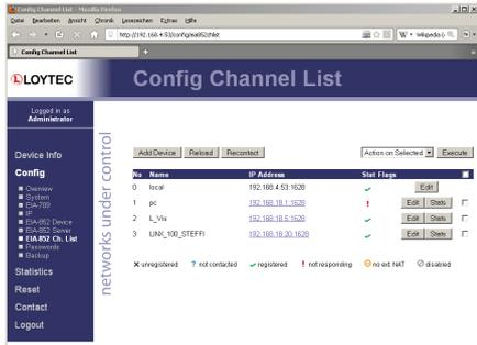
Besides the router functionality, the L-IP Routers provide outstanding capabilities for network diagnostic and analysis. They allow the LPA (LOYTEC Protocol Analyzer) transparent access to the twisted pair channels (TP/FT-10 or TP/XF-1250) on the device via Ethernet/IP – via a local Intranet or the Internet. This allows a fast analysis of data communication and reduces time-consuming troubleshooting. All system registers are available as OPC XML-DA and OPC UA data points.
