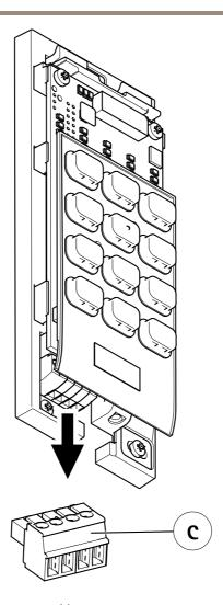
5. Remove the connector head (c) and connect the wires. For connector specifications, see *Power & Data Connector on page 10*.
