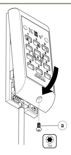
8. Hook the frontplate onto the upper tabs on the backplate, push the frontplate into place and tighten the screw (a).
