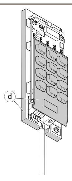
7. Check that the silicone gaskets (d) fit tightly to the backplate sides and over the keys.
