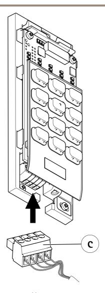
6. Reattach the connector head (c).
