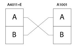
To use the reader with AXIS A1001, connect the RS485 wires from A to B and from B to A.
