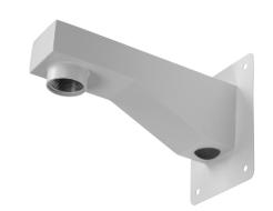
The **IDM4012SS** wall mount is designed specifically for the Stainless Steel and Pressurized Spectra<sup>®</sup> Series Dome Systems (Spectra III<sup>™</sup> or newer models). The mount is constructed of type 304 stainless steel with a gray polyester powder coat finish making it ideal for harsh environmental installations.
