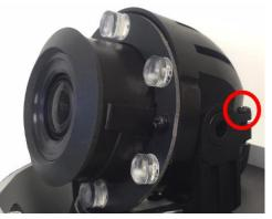
7. Install the dome lanyard if removed and then the dome cover and tighten the dome cover screws.
