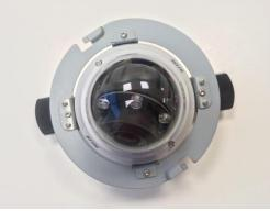
12. Put on the trim ring and rotate it clockwise to secure the trim ring on the bracket.
