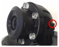
10. Install the dome lanyard if removed and then the dome cover and tighten the dome cover screws.
