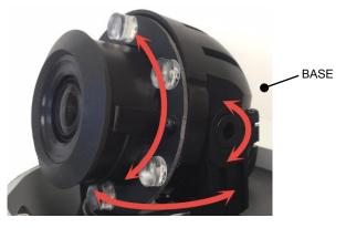
5. Tighten the locking screw to secure the camera module position.
