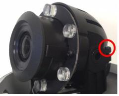
11. Secure the anti-drop chain, put on the dome cover, and tighten the dome cover.
