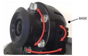
9. Tighten the locking screw to secure the camera module position.
