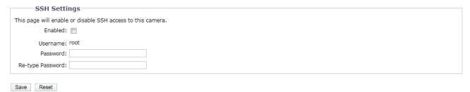
FIGURE 3-17: ENABLING SECURE SHELL
