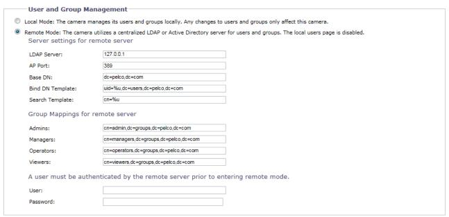
FIGURE 3-39: ENABLING REMOTE MODE
