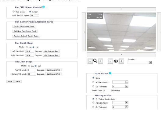
FIGURE 3-32: Positioning Settings
