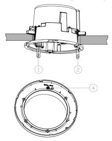
FIGURE 2-15: Attaching the Lower Dome
