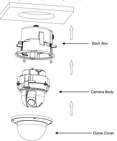
FIGURE 2-16: OUTDOOR IN-CEILING INSTALLATION
