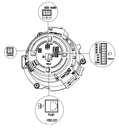
FIGURE 2-2: CONNECTORS FOR WIRING
