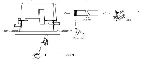
FIGURE 2-13: OUTDOOR IN-CEILING CABLING
