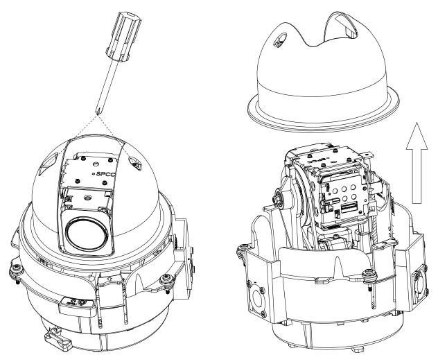
FIGURE 2-1: DISASSEMBLE THE CAMERA
