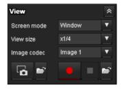
You can change the screen mode, view size of the image, image codec mode and frame rate. Also, still images and movies can be saved (movie saving can also be stopped) from here. Microphone and audio output levels can be adjusted.
