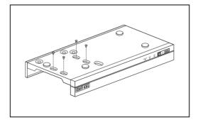
**4.** Check for any problems in the connection terminal and the wiring in the product, close the cover and fix it with screws.
