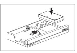
**3.** Using the screws, fix the HDD to the bottom of the set.
