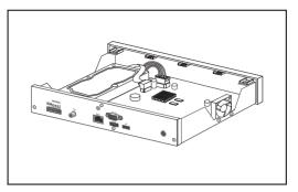
5. Close the cover, and tighten a setscrew in the back.
